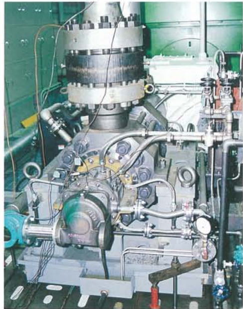
Segmental ring-section casing boiler feed pump 9,310ft-3,114 U.S.gpm-5,840min -1 -9,650HP
