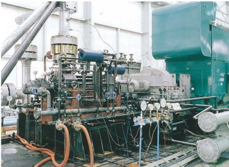
Segmental ring-section boiler feed pump 2,720psi-2,430U.S.gpm -6,060min -1 -5,360HP Bin Qasim Power Plant(Pakistan) , 210MW×1units
